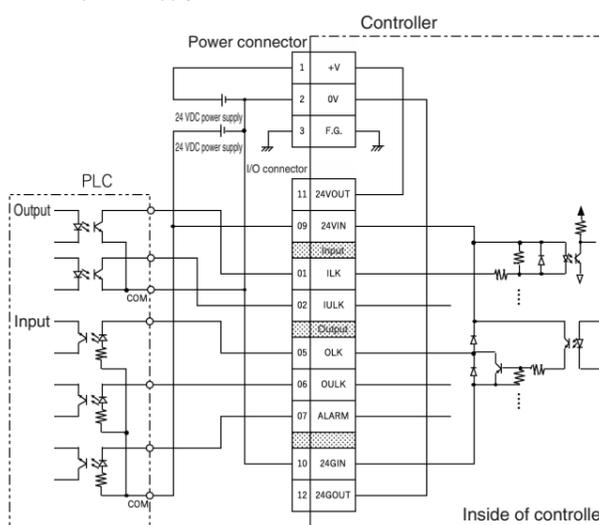
\* Even when using just input or output, connect power to 09 and 10.
