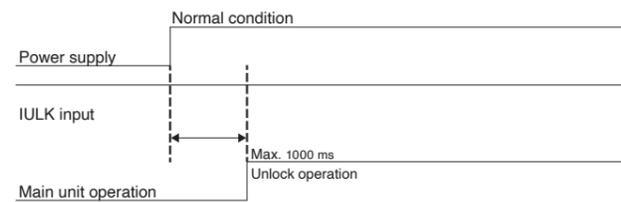
\* When "Controller SW1: OFF state", then operation starts according to IULK signal when power is turned ON.
