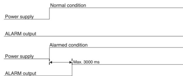
\* Before operating, confirm that the ALARM output does not turn ON after the power is turned ON.
