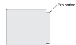
\* To remove the protective front cover, hook your finger on the projection on one side of the cover and remove it.
