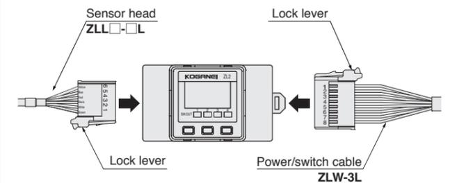
To attach the sensor head and the power/switch cables, position the lock levers as shown in the illustration above, and then insert until they lock into place with the controller side connectors. To disconnect, press the lock lever down as far as it will go as you pull the connector to unplug it. At this time, take care not to apply undue force to the lead wires.
