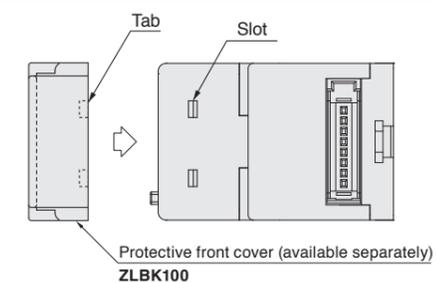
Attach the protective front cover so the tabs inside the cover enter the slots on the Linear Magnetic Sensor Controller.
