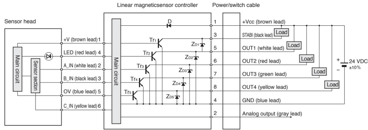
Note: Note that extending the cable can cause a drop in voltage due to cable resistance.
