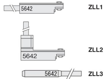
Refer to the parameter code embossed on the sensor head, and follow the example below to enter the parameter code. The parameter code is embossed at the position shown in the sensor head diagrams on the right with the format display side facing up.
