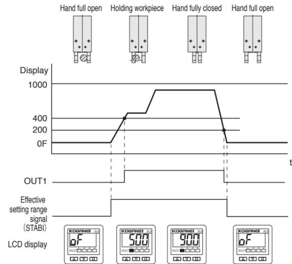
CAUTION: When the effective measuring range signal is OFF (outside the measuring range), OUT also becomes OFF.
