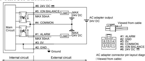
Note1: GND is connected internally to 0V.
