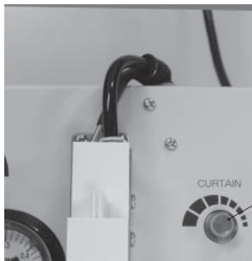
Throttle valve for air curtain
