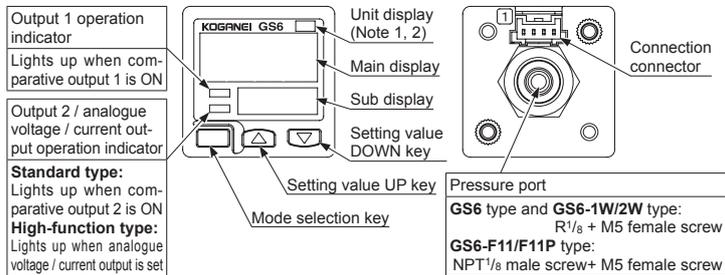
Notes: 1) In the case of a model that is intended for use outside Japan, attach the unit switch plate corresponds to the set pressure unit.
