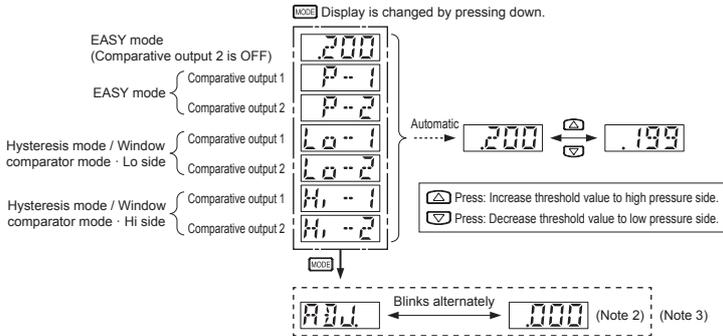
Notes: 1) If the set pressure range is exceeded, "UP" (exceeds the upper limit) or "DOWN" (exceeds the lower limit) will appear on the sub display. "DOWN" will also appear if the Hi side threshold value exceeds the Lo side threshold value when setting the "hysteresis mode / window comparator mode" threshold value.
