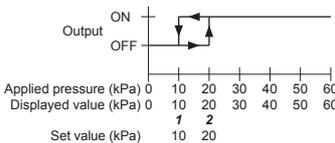
**During remote zero-adjustment input**
