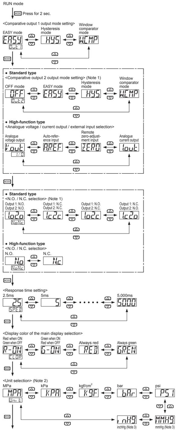
Notes: 1) If the comparative output 2 output mode setting is set to "OFF", the display of N.O. / N.C. selection is the same as the high-function type.
