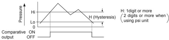
Note: "H<sub>1</sub> - 1" or "Lo - 1" is displayed for comparative output 1 and "H<sub>2</sub> - 2" or "Lo - 2" for comparative output 2 on the sub-display.
