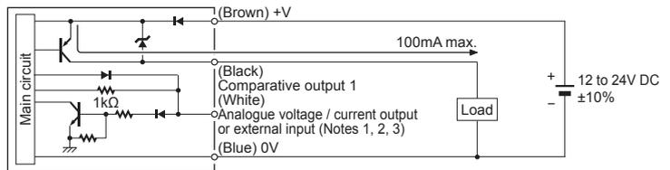
Notes: 1) When the analogue current is output, the output load resistance should be 250Ω max.
